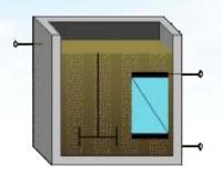
**Moving Bed Biofilm Reactor** - An MBBR unit process has been added that supports BOD removal and nitrification. The user can now compare the cost differences between the conventional and the media based process technologies. The MBBR cost analysis includes the costs of the screens, media, tanks, blowers, energy and labor.
