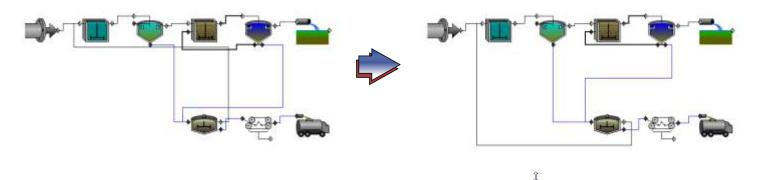
**Custom Process Images** – To distinguish between similar processes or to make a more visual link between the actual plant and the CapdetWorks representation, the user can now replace the default process images with pictures of their actual unit processes.
